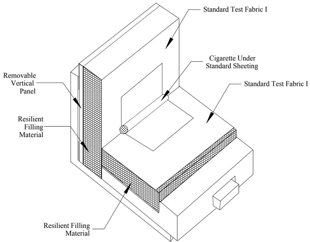
Figure C-5. Decking Materials Tester.
