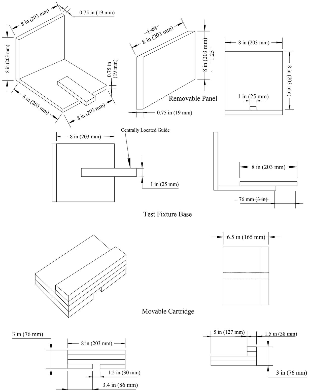
Figure C-2. Mock-up Assembly for Smoldering Ignition Resistance Test of Upholstery Cover Fabrics
